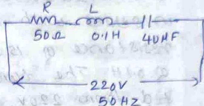
$$X_C = \frac{1}{\omega C} = \frac{1}{2\pi f C} = \frac{1}{2\pi \times 50 \times 40 \times 10^{-6}} \Omega$$
